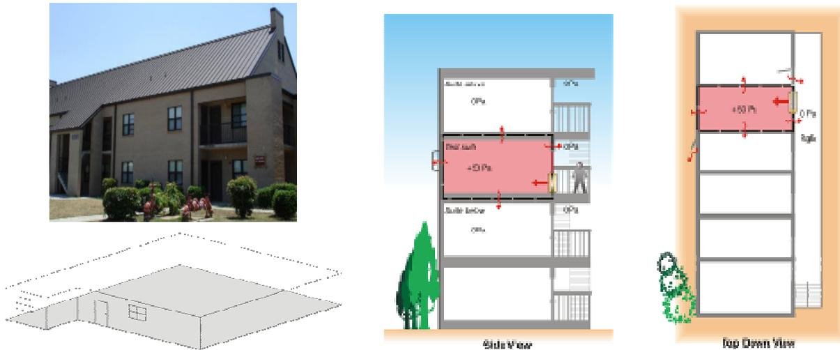
**Figure 2. Example building where individual apartments have doors to the outside**
