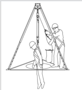
The SuretyMan Rescue Utility System can be used in conjunction with the Sure-Strong Tripod
