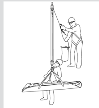
The SuretyMan Rescue Utility System can be used in conjunction with the Sked Rescue system
