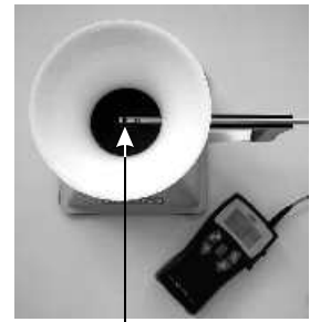
Position the hot-wire probe
