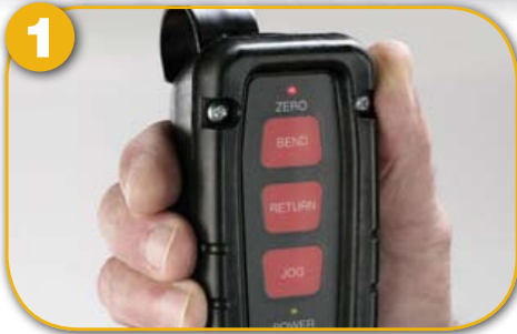
NEW Ergonomic Pendant Control Ease of operation
