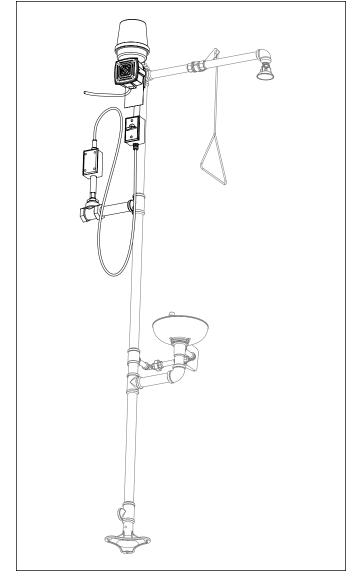
This Alarm System is designed to meet NEMA NO. 3R Code (WATERPROOF).
