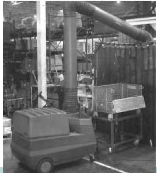
the fume to move more quickly to the filters, it was still passing through the welder's breathing zone.
