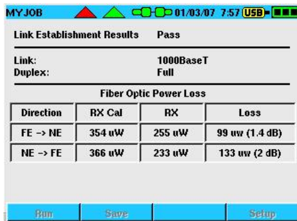
Figure 6-6 Fiber Link Establishment
