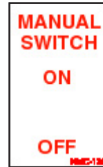
Manual switch (Bypasses remote)
