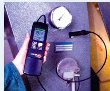
Measuring the CO 2 conc. in ingoing and outgoing air ducts
