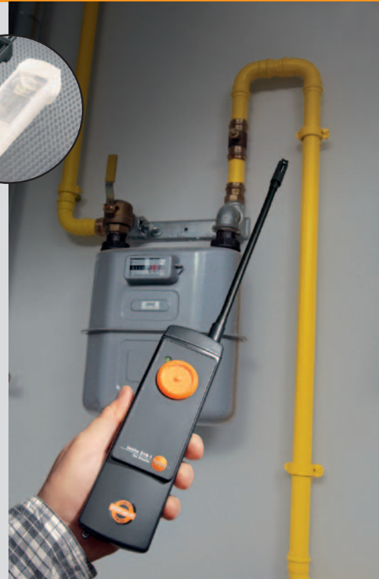
Checks for leaks in domestic gas pipes
