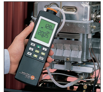
Checks gas flow pressure
