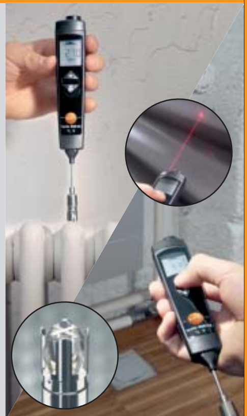
Temperature measurement on a non-smooth radiator using a self-adapting, flexible measuring head and non-contact measurement on a radiator
