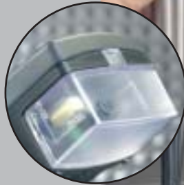
Condensate trap in instrument
