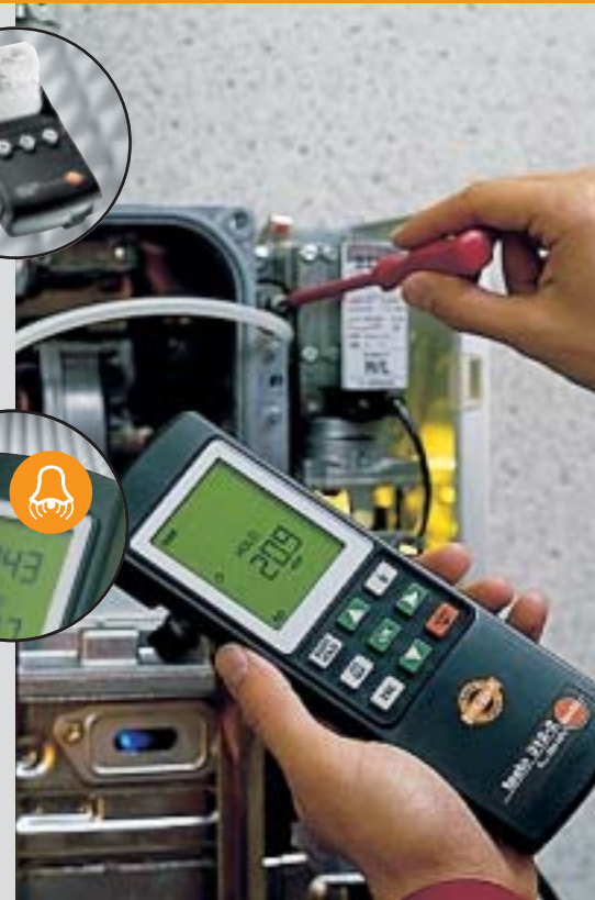
Differential pressure measurement on heating units
