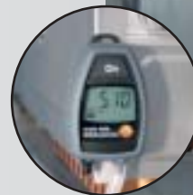
Electronic U-tube manometer
