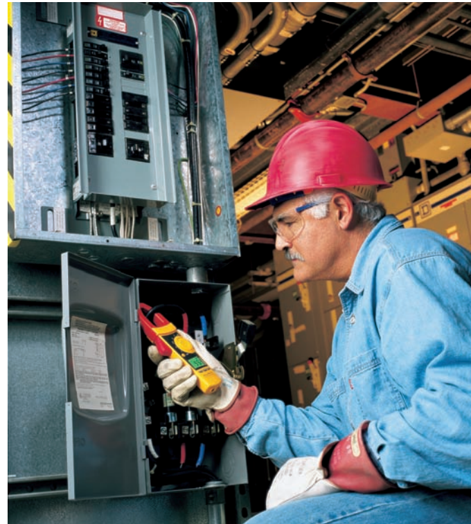
Choose a clamp meter rated to meet the electrical environment you'll be working in, as well as the resolution and accuracy of measurement you'll need for your testing.
