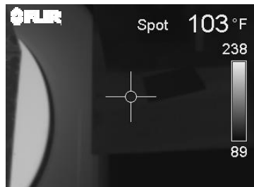
Figure 6.3: Room temperature aluminum, apparent temperature, 103°F
