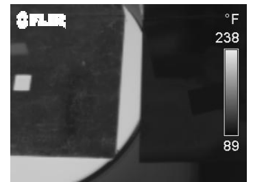
Figure 6.4: Comparison of hot aluminum (left) and room temperature aluminum (right)
