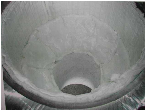
Figure 12. Close-up view of new cylinder and bowl gasket design
