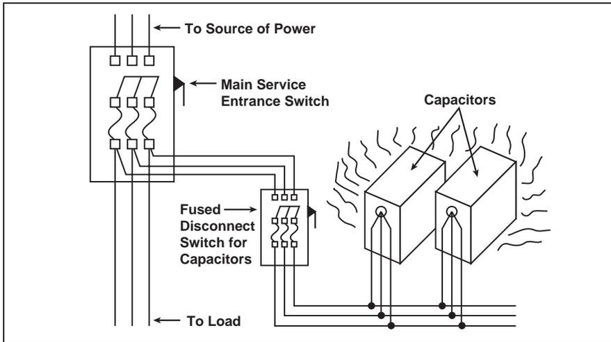
Figure 10. Power factor capacitors at resonant frequency.
