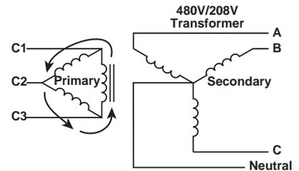
Figure 9. Delta primary, circulating current
