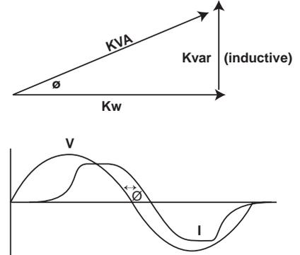
Figure 5. Power factor on nondistorted sine wave.
