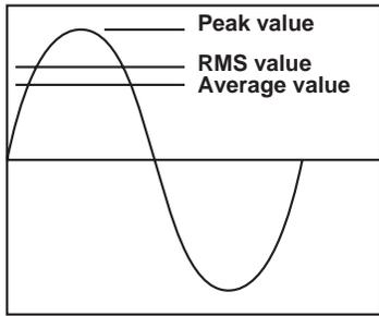
Figure 12. RMS – Avg – Peak Relationship in sine wave
