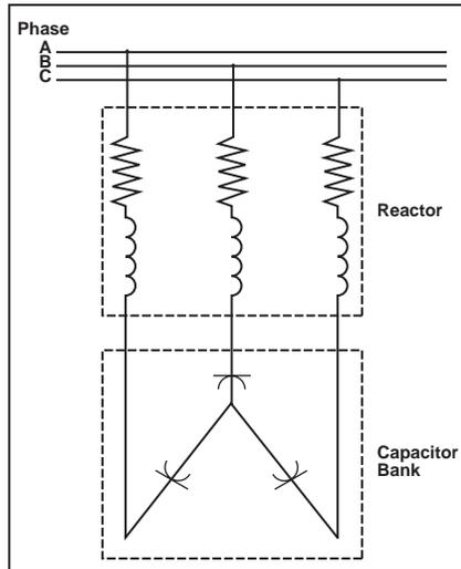
Figure 13. Single tuned shunt filter.
