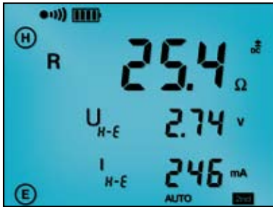
The 4-Point Bond test displaying lead connections, bond resistance test results, test voltage and current.
