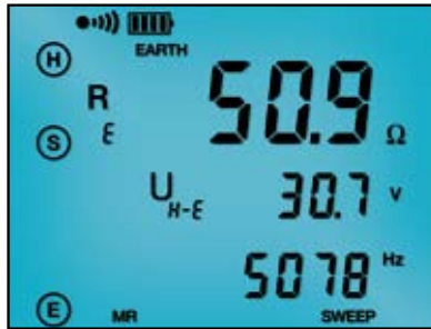
The 3-Point Fall-of-Potential test displaying test lead connection, grounding electrode resistance, test voltage and frequency.
