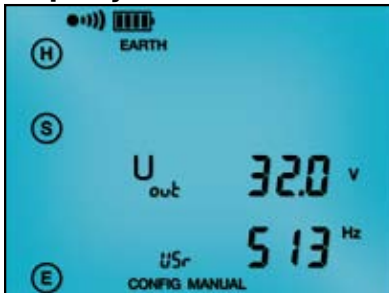
The Frequency selection screen displays selected test frequency and voltage for the test as well as lead connection.
